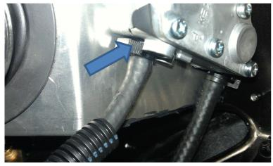
We suggest replacing impulse line with a 2" longer line
