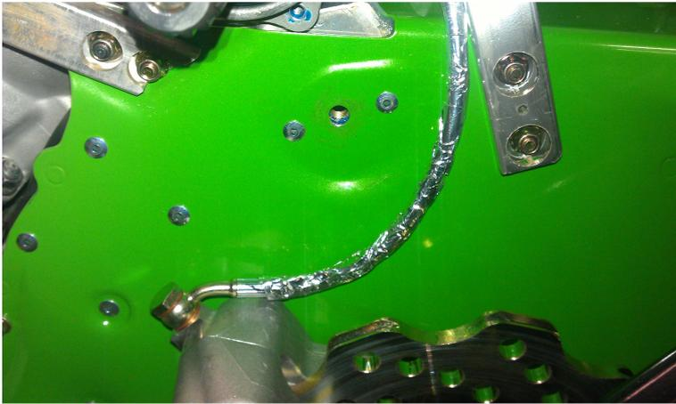
Might be a good idea to install some heat foil tape and or heat loom in that area 6' to 8" from the crimp fitting up. Make sure to inspect it closely if you have really got the brake pads and or the fluid hot at any point.
